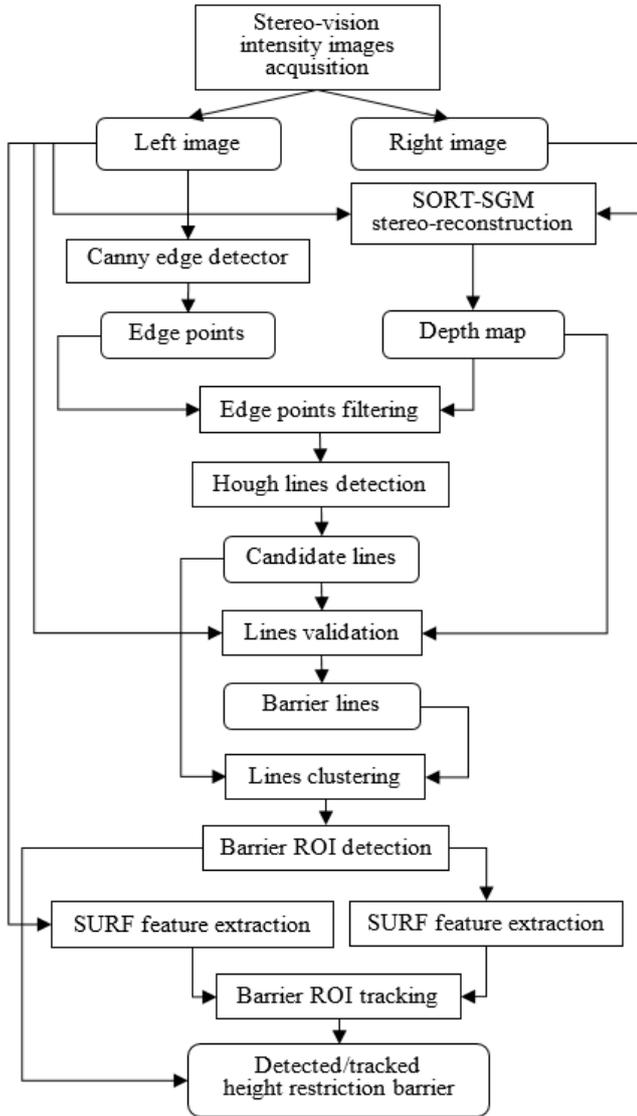
Figure 2. Height restriction barriers detection and tracking system architecture
